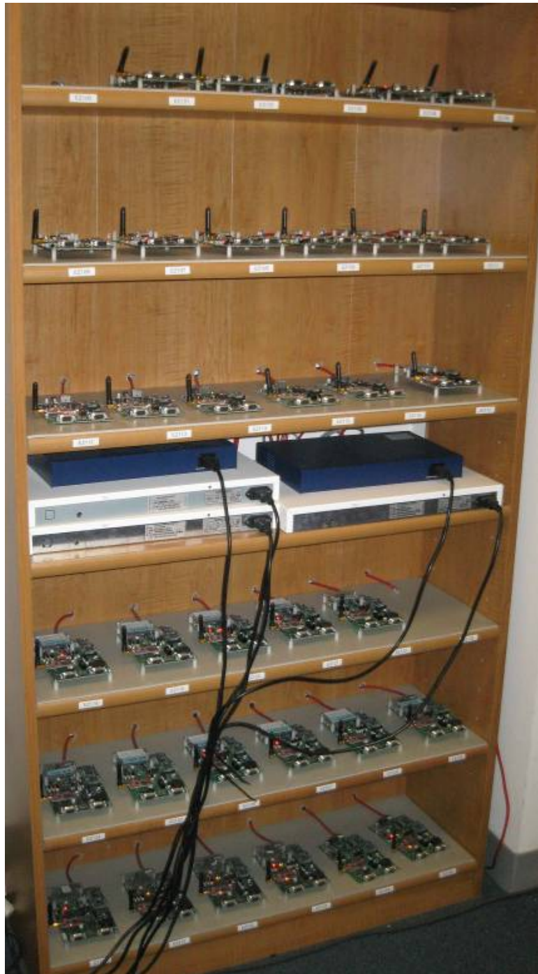
Figure 2-4. 36-Node Density Test Setup
